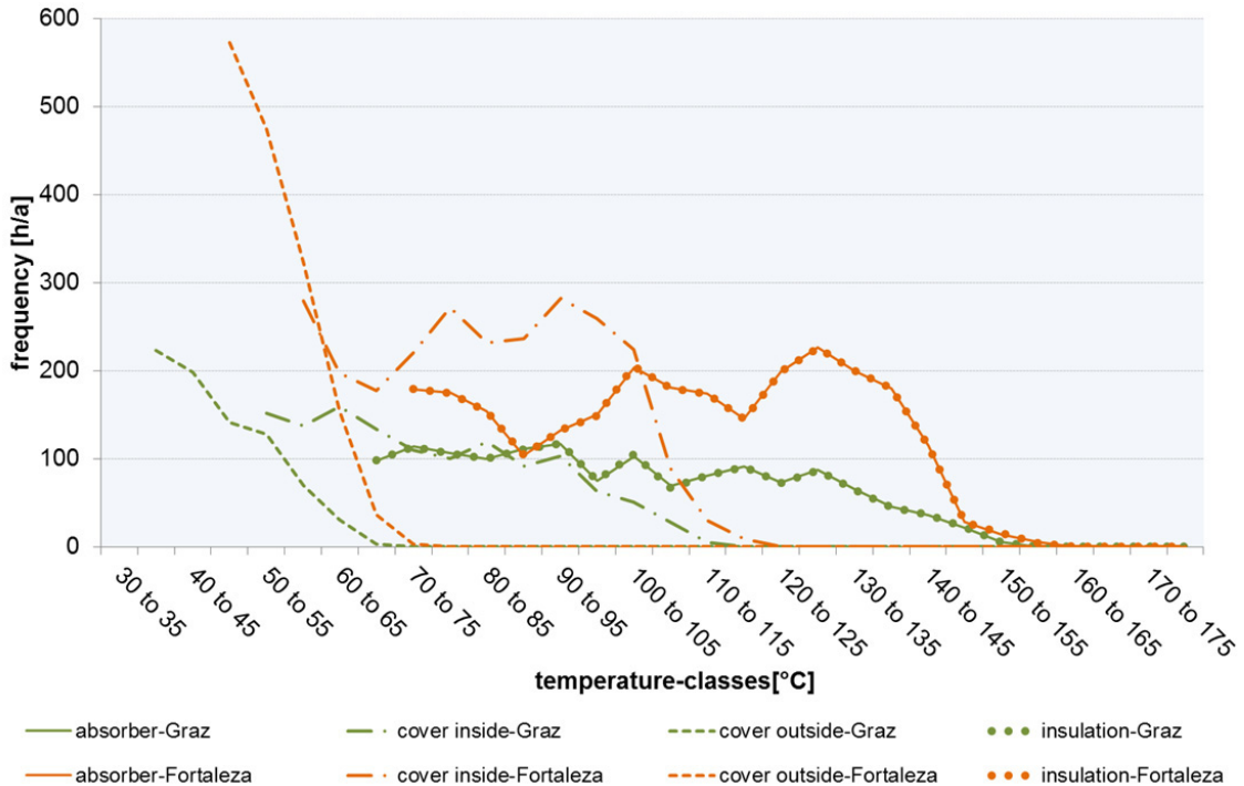
Fig. 5. Annual frequencies of temperature stress of different components in plastic panels (plastic cover, plastic absorbers, insulation) in the unfilled system state (maximum load) for the locations Graz and Fortaleza. Only irradiation values greater than 300 \text{ W / m}^2 were taken into account.
